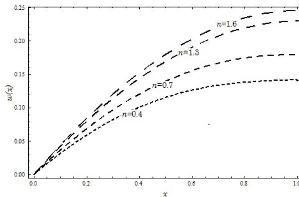
**Figure 2.** Profiles of the Sisko fluid film velocity, for various values of fluid behaviour index  $n$  when  $S_f = 0.6$  and  $\beta = 0.4$ .
