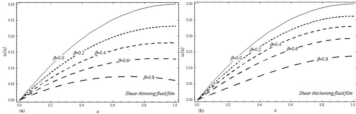
**Figure 3.** Profiles of the velocity, for various values of Sisko fluid parameter  $\beta$  when  $S_f = 0.6$ , (a)  $n = 0.7$  and (b)  $n = 1.3$
