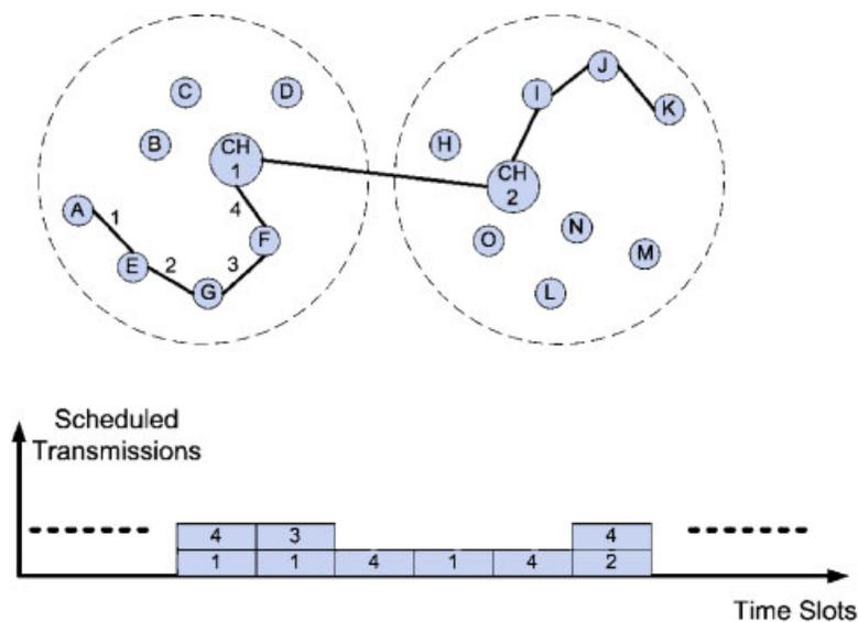
Fig. 1. A clustered TD/CDMA wireless ad hoc network. CH, cluster head.
