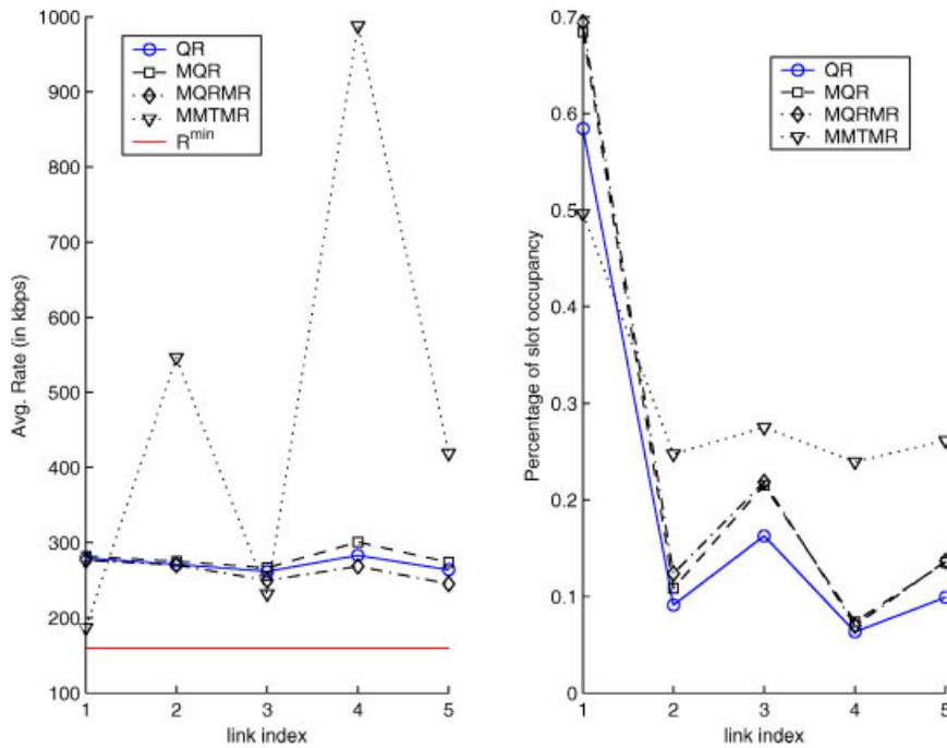
Fig. 5. Comparison of throughput-optimal family of algorithms in a linear TD/CDMA wireless ad hoc network.
