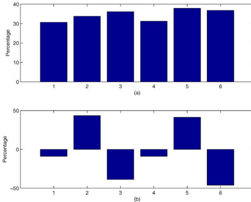
Fig. 9. Gain/loss of distributed algorithms over their centralized counterparts: (a) Total average rate, (b) Effective rate. 1, MPFMR ( $r_{II}$ ); 2, MQRMR ( $r_{II}$ ); 3, MPFMR ( $r_{III}$ ); 4, MQRMR ( $r_{III}$ ); 5, MPFMR ( $r_{IV}$ ); 6, MQRMR ( $r_{IV}$ ).
