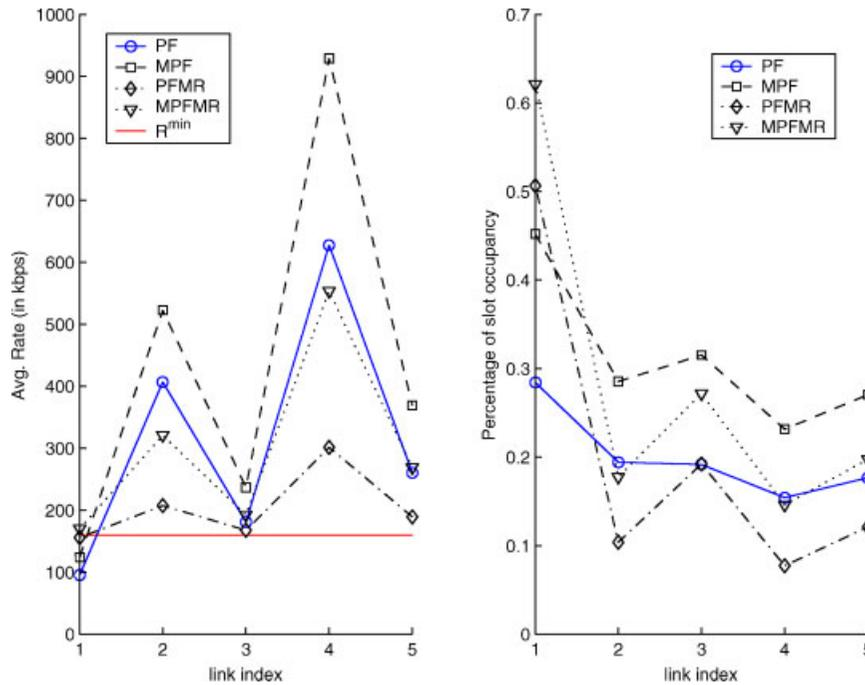
Fig. 4. Comparison of PF-family of algorithms in a linear TD/CDMA wireless ad hoc network.
