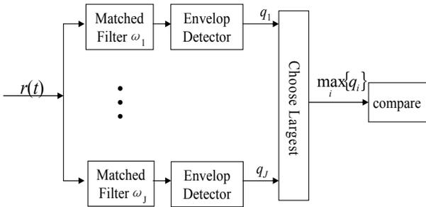
Figure 1. The block diagram of the subcarrier detector
