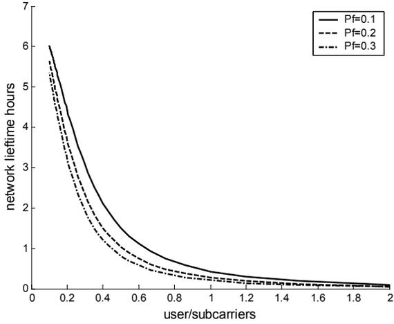
Figure4. Impact of user/subcarriers and false alarm probability  $P_f$  to lifetime
