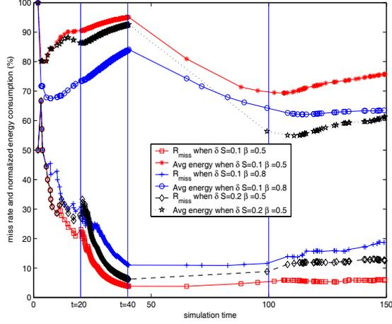
Fig. 5. event miss rate and normalized average energy consumption using the proposed AT scheme with different parameter settings.
