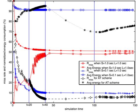
Fig. 4. event miss rate and normalized average energy consumption using 2 FT schemes and the proposed AT scheme (with  $\delta S = 0.1$  and  $\beta = 0.5$ ).
