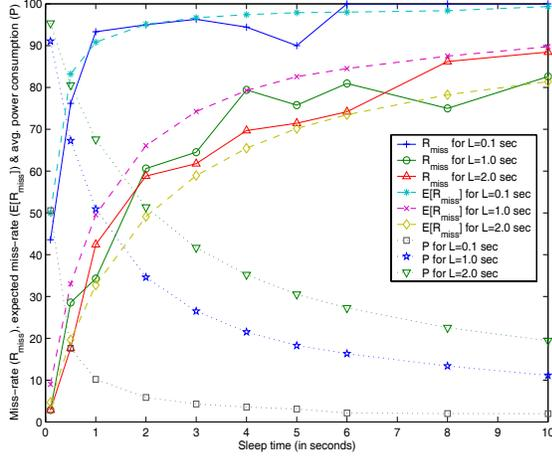
Fig. 2. event miss rate and normalized average energy consumption vs. sleep time when the Poisson rate of events and listen intervals are fixed.
