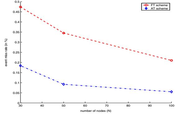
Fig. 7. event miss rate vs. number of sensor nodes in the network ( $r$  is fixed,  $r=15m$ )
