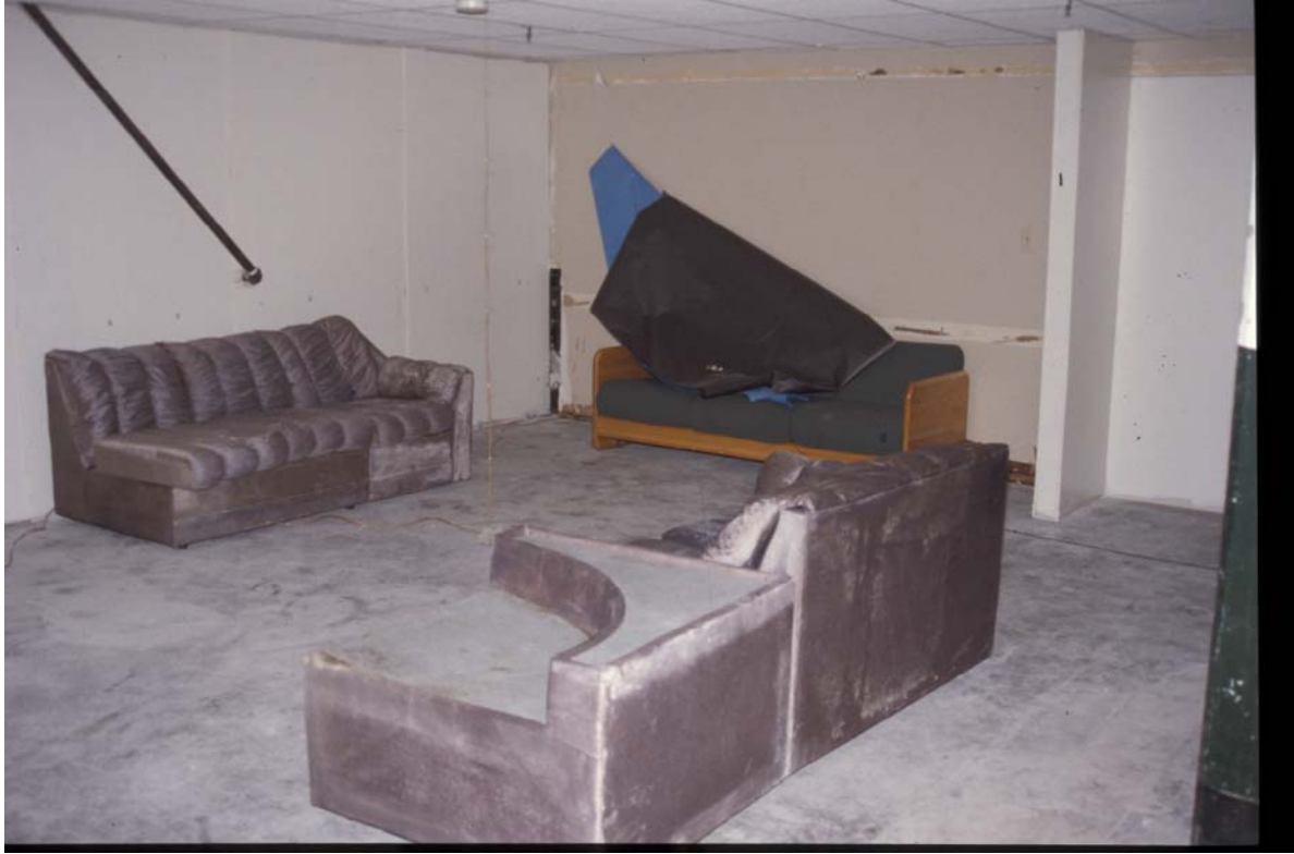
Figure 6. Photograph showing the fuel arrangement for the day room in experiment 1.
