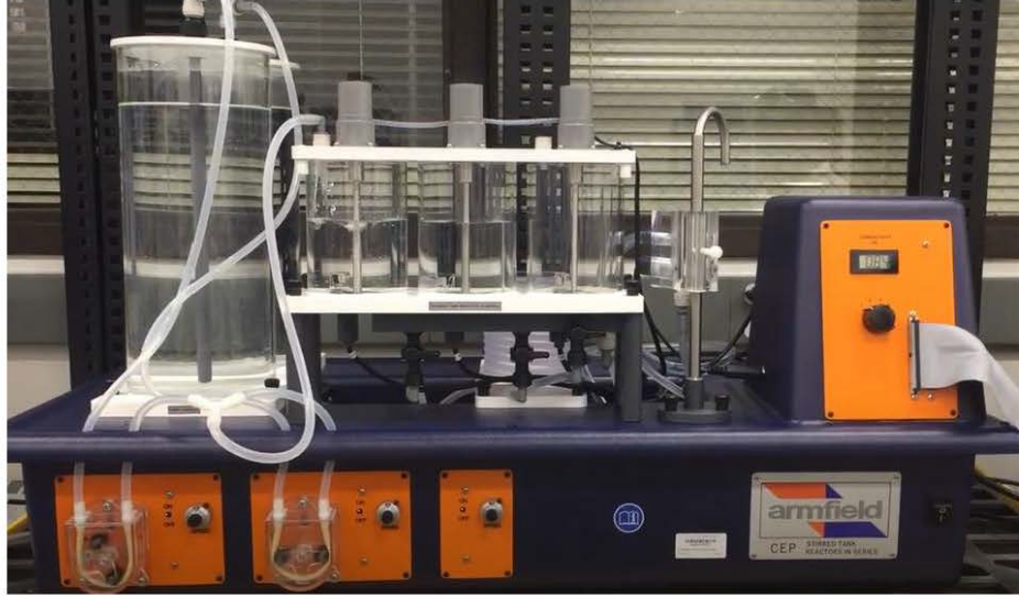
Figure 2: CEP-MkII Stirred Tank Reactors in Series
