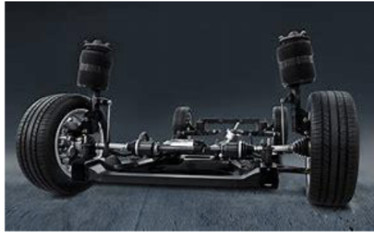
Figure 3 AIRMATIC Suspension on Mercedes-Benz CL-Class
