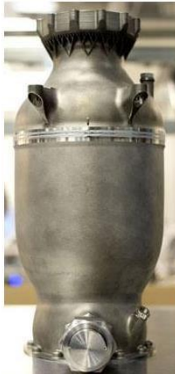
Figure 1.3 – SuperDraco printed engine chamber [9]
