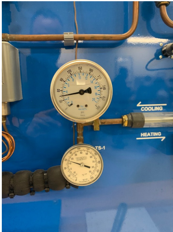
Figure 1.7 Example Temperature and Pressure Gauges of Amatrol T7082
