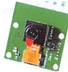
5.2: Raspberry Pi Camera Rev 1.3
