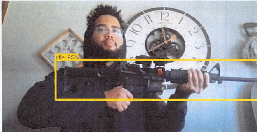
Figure 12.1: Rifle Detected with 95% Confidence
