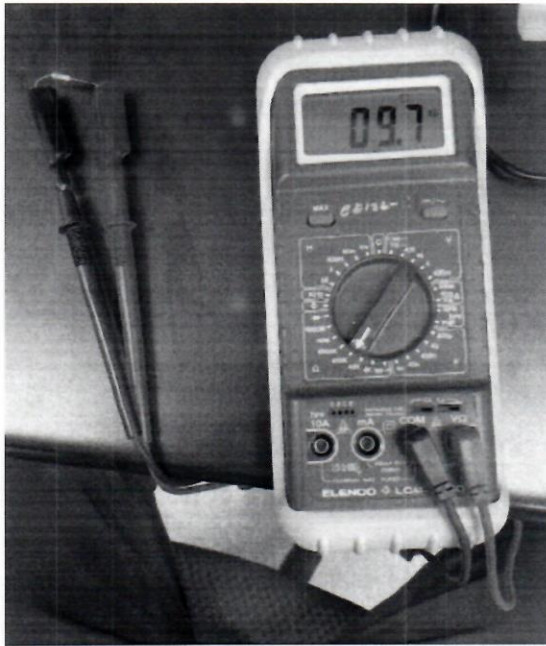
Figure 5: 1K Resistor measured by Multimeter
