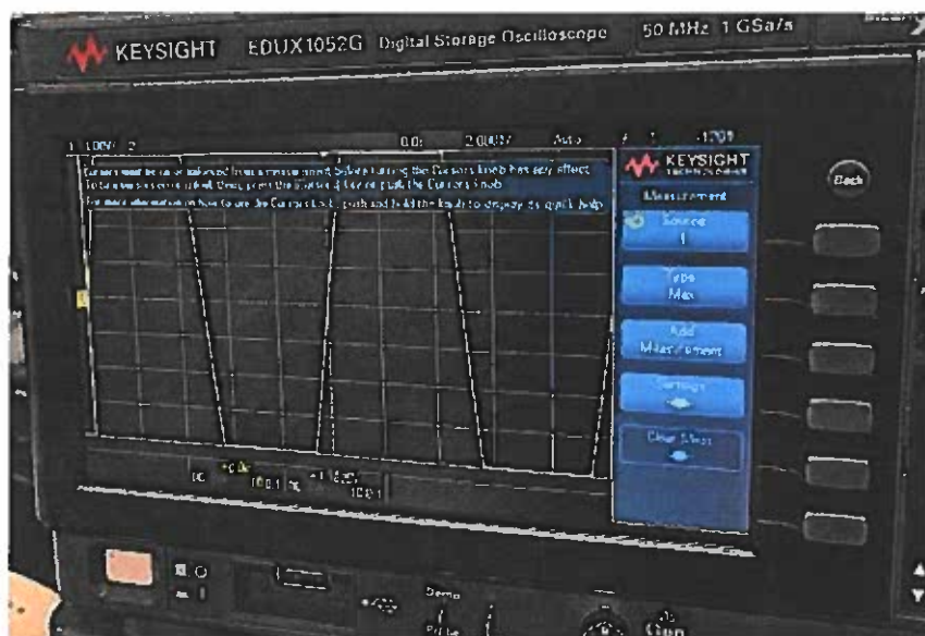
Figure 9. Inverting Amp Graph(100kohm resistor)
