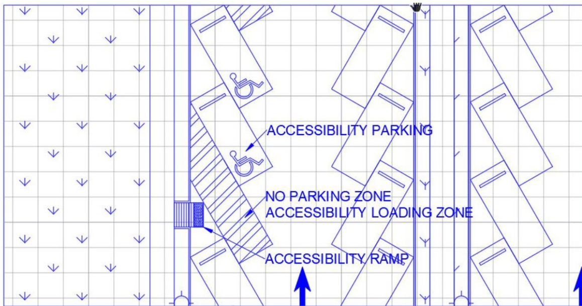
TYPICAL ACCESSIBILITY MARKING DETAIL
