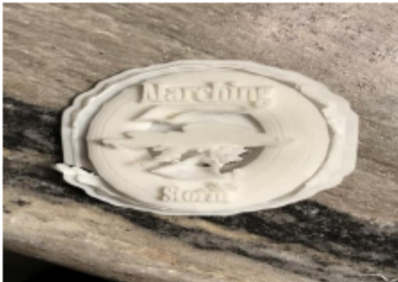
Figure 2. 1 st Attempt at Removing Supports
