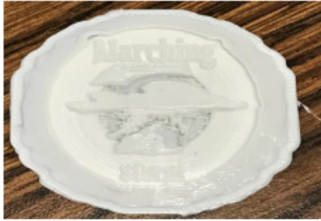
Figure 4. 1 st Design with Full Supports
