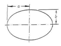
$$\begin{split} A &= \pi a b \\ p_{\rm approx} &= 2 \, \pi \sqrt{(a^2 + b^2)/2} \\ P &= \pi (a + b) [1 + ({}^1\!/_2)^2 \lambda^2 + ({}^1\!/_2 \times {}^1\!/_4)^2 \lambda^4 \\ &+ ({}^1\!/_2 \times {}^1\!/_4 \times {}^3\!/_6)^2 \lambda^6 + ({}^1\!/_2 \times {}^1\!/_4 \times {}^3\!/_6 \times {}^5\!/_8)^2 \lambda^8 \\ &+ ({}^1\!/_2 \times {}^1\!/_4 \times {}^3\!/_6 \times {}^5\!/_8 \times {}^7\!/_{10})^2 \lambda^{10} + \dots ] \,, \end{split}$$
