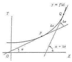
The curvature K of a curve at P is the limit of its average curvature for the arc PQ as Q approaches P. This is also expressed as: the curvature of a curve at a given point is the rate-of-change of its inclination with respect to its arc length.
