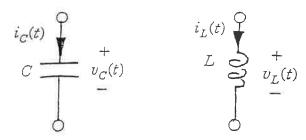
The charge  $q_{\mathcal{C}}(t)$  and voltage  $v_{\mathcal{C}}(t)$  relationship for a capacitor C in farads is
