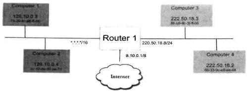
(4 pts) (5.1) Assign an IP address to the leftmost interface of <u>Router 1</u>, given that the NetID part of IP addresses are 16 bits (or slash notion /16).
