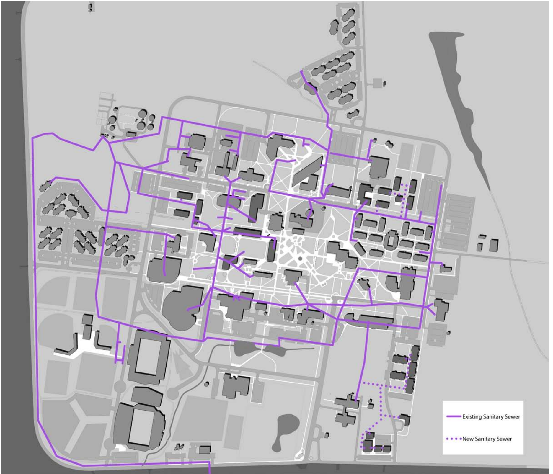
Figure 3.6: Sanitary Sewer Plan
