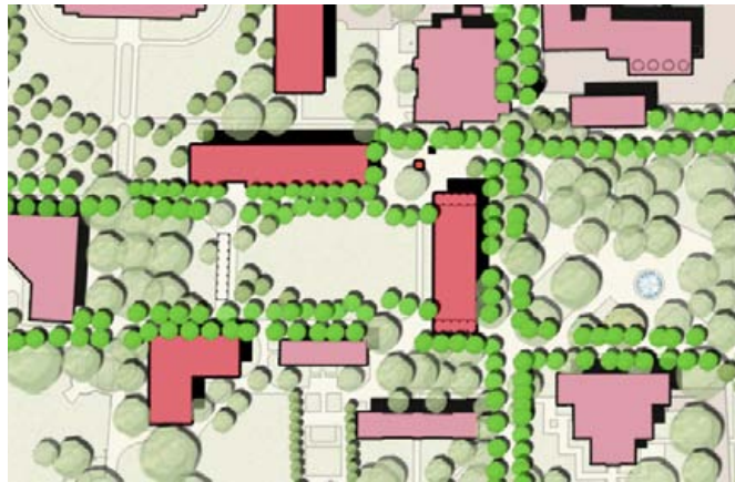
Figure 1.23: Primary walks with continuous rows of shade trees of a single species.
