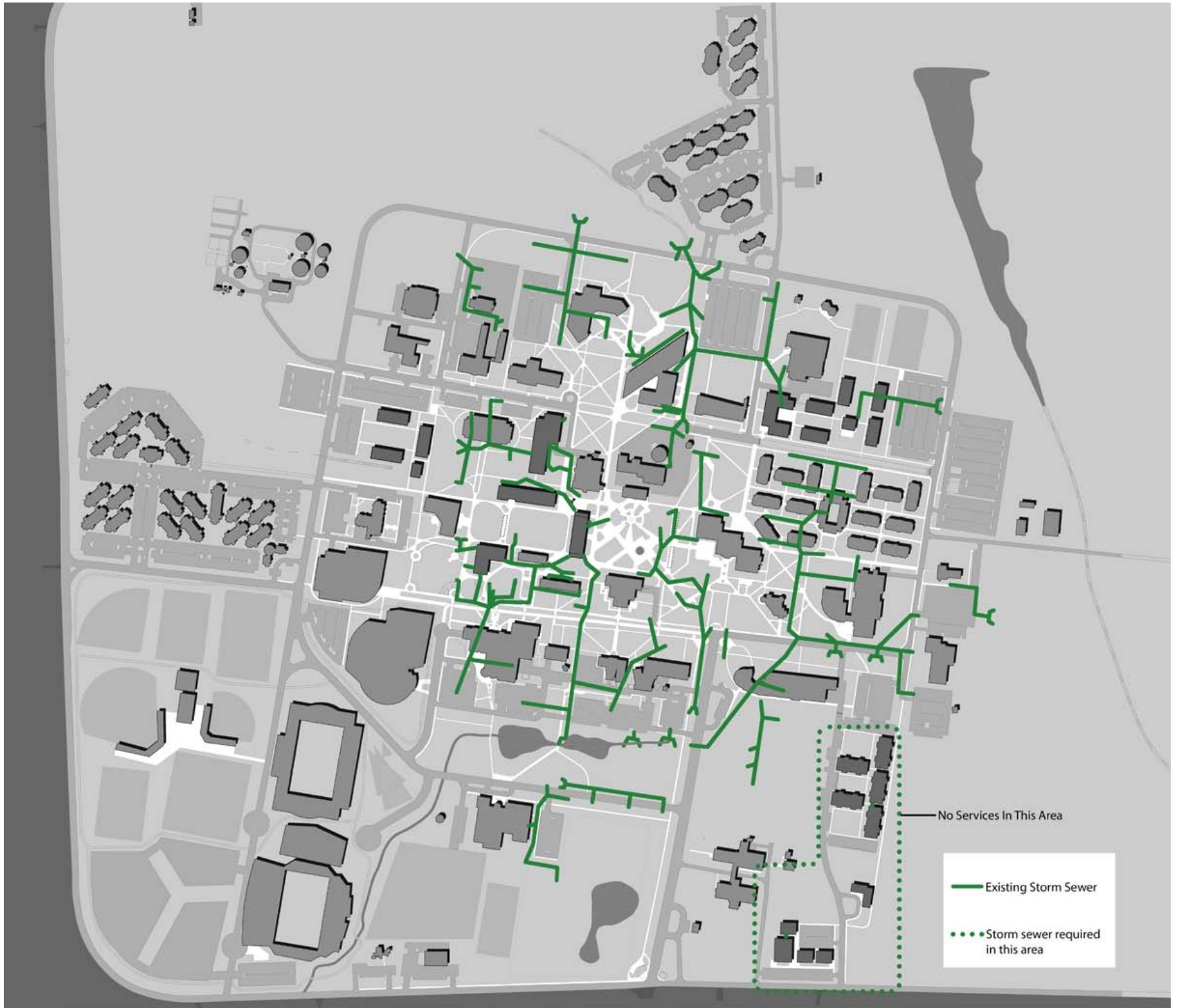
Figure 3.5: Storm Sewer Plan
