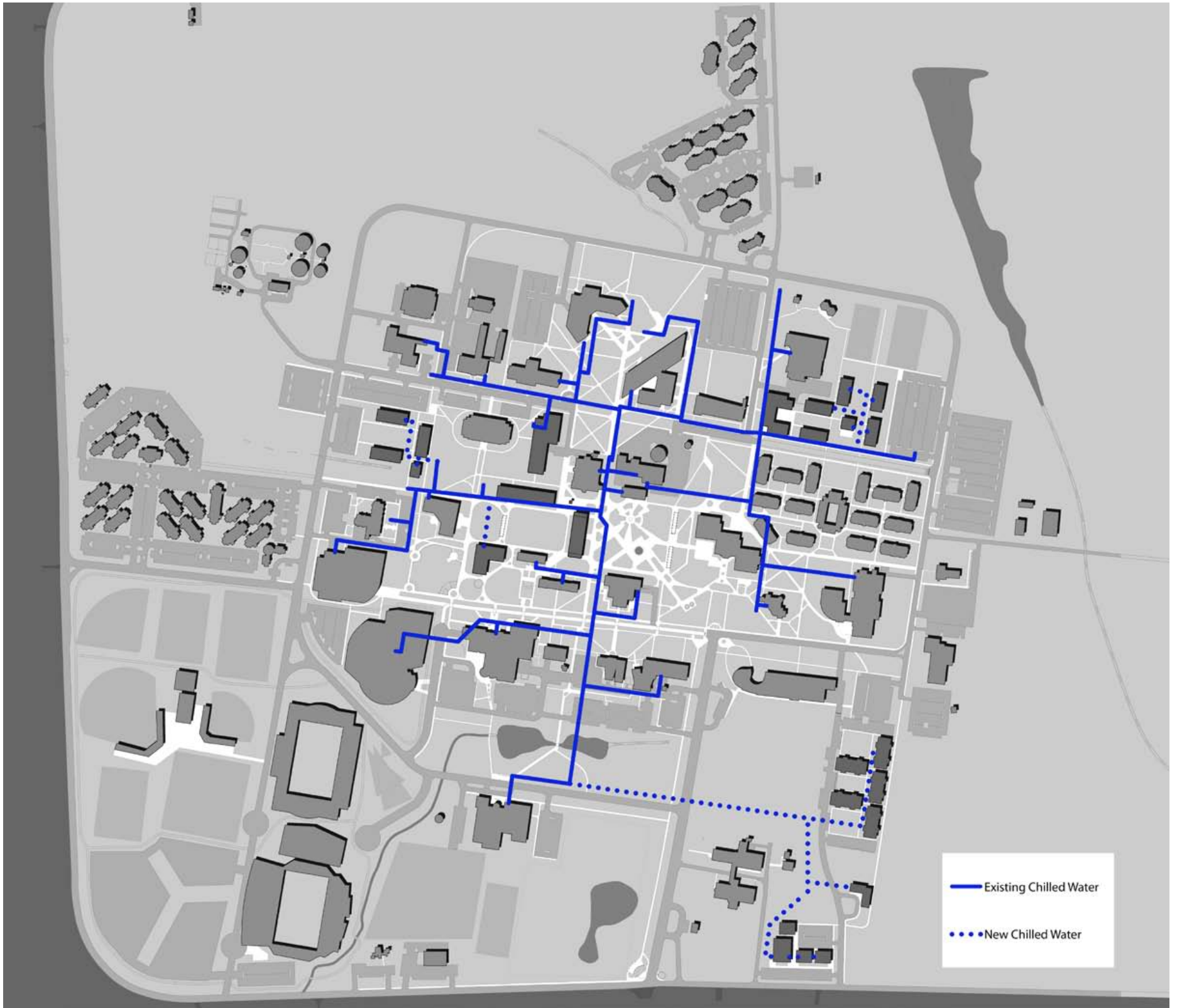
Figure 3.3: Chilled Water Plan
