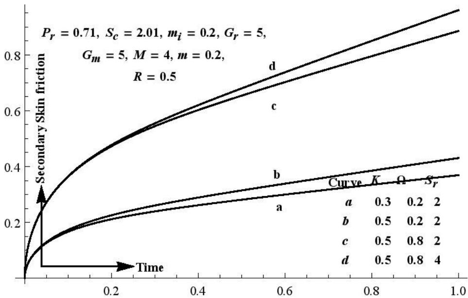
Figure 9. Secondary skin friction  $K, \Omega$  and  $S_r$  in case 1
