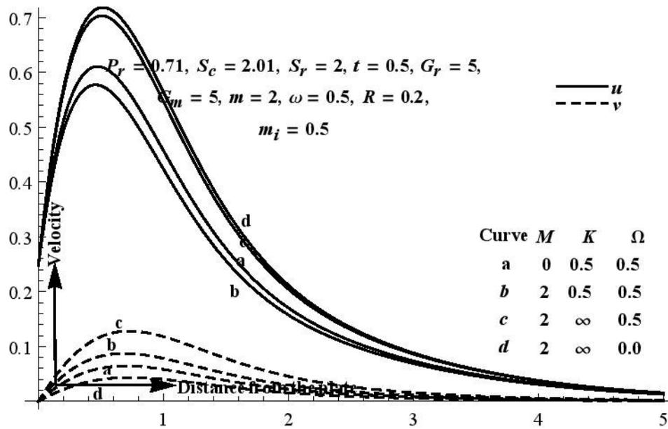
Figure 6. Velocity profile for  $M, K$  and  $\Omega$  in case 2
