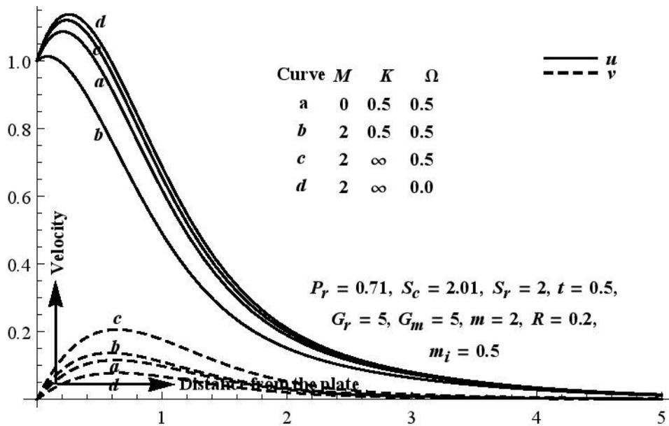
Figure 5. Velocity profile for  $M, K$  and  $\Omega$  in case 1
